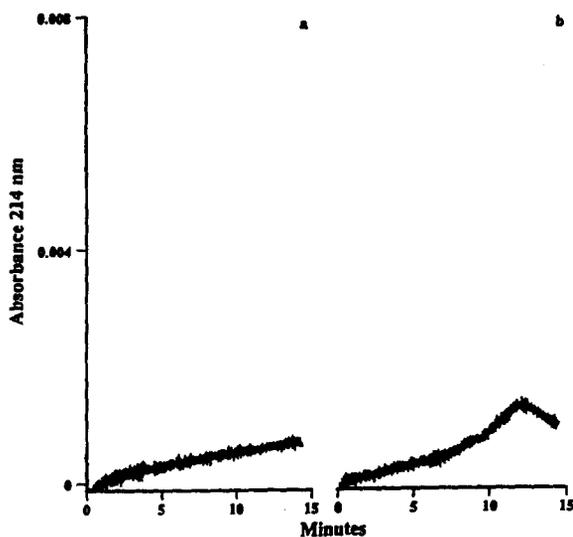
Fig. 2. Electropherograms of the enzymes neuraminidase and  $\beta$ -N-acetyl glucosaminidase. The capillary was 57 cm  $\times$  75  $\mu$ m I.D. and the separating voltage was 20.5 kV. UV absorbance was measured at 214 nm. The sample loaded into the capillary was 30 nl. A Beckman P/ACE was used. (a)  $\beta$ -N-Acetyl glucosaminidase; (b) neuraminidase.
